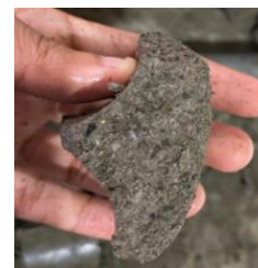
Fig. 2 Properly mixed geopolymer binder and soil
