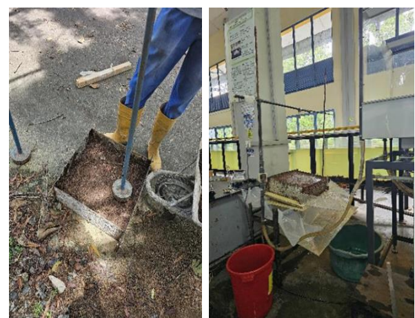
Fig. 2 Sample Preparation and the Erosion test
