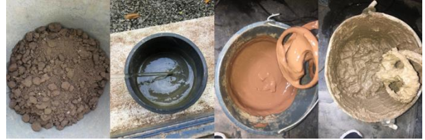
Fig. 2 Used soil, cement grout, bentonite slurry and prepared SCB backfill in the order
