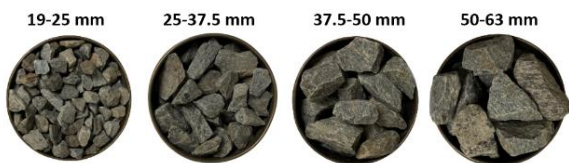
Fig. 2 Ballast Particles size ranges
