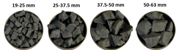
Fig. 3 Rubber Particles size ranges
