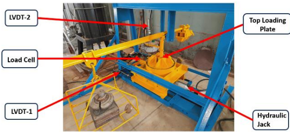
Fig. 5 Large scale direct shear test apparatus
