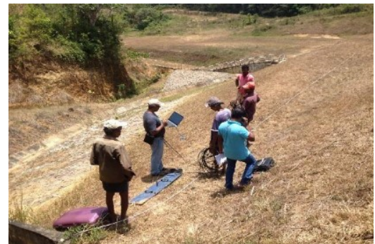
Figure 2 : GPR survey – Kekiriobada dam
