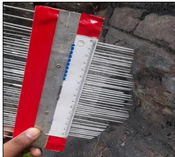
Fig. 2 Self-fabricated 15cm Barton's comb profiler
