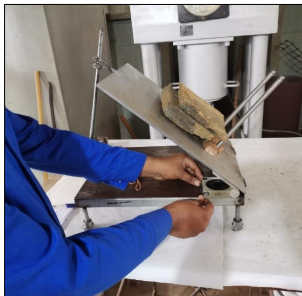
Fig. 3 Self-fabricated tilt test apparatus to determine the peak friction angle.
