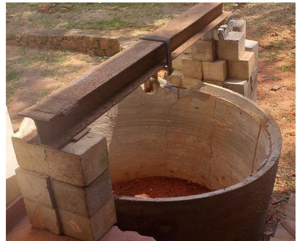
Fig.2 Arrangement for dynamic compaction
