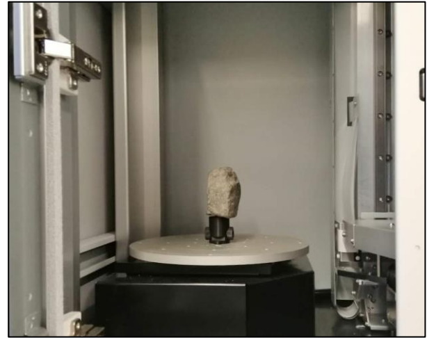
Fig. 2: 3d Scanning of Actual Ballast Particle
