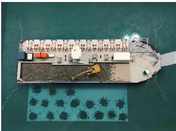
Fig. 4 Barge section during geotextile placement
