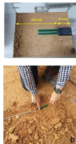
Fig. 8 Soil moisture sensor and its installation
