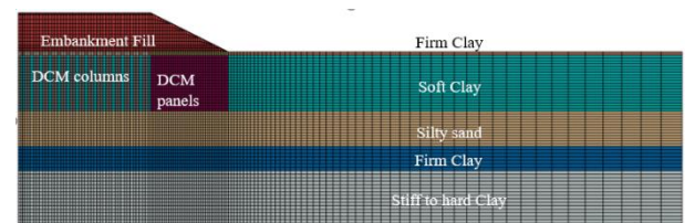
Figure 3: Finite element model of the case study
