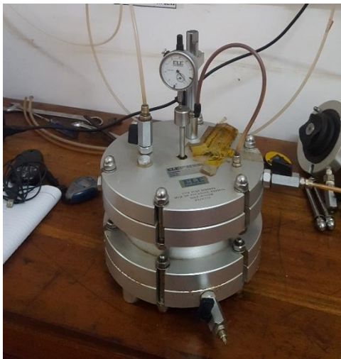
Fig.4 Sample loaded in the Rowe cell
