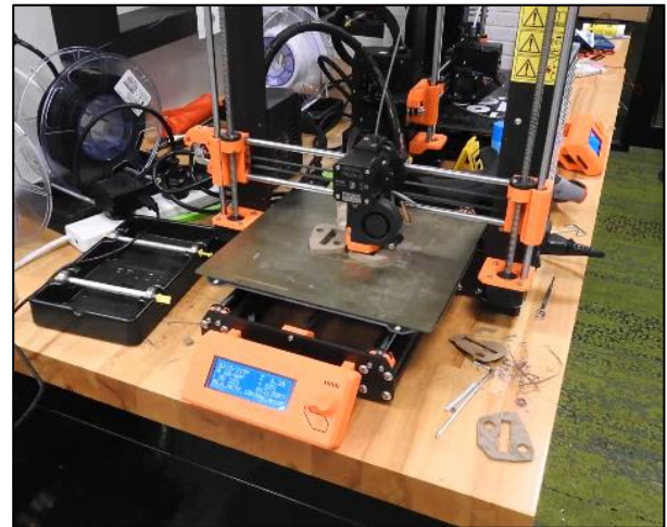
Fig. 3: 3d Printing of Smart Ballast Particle
