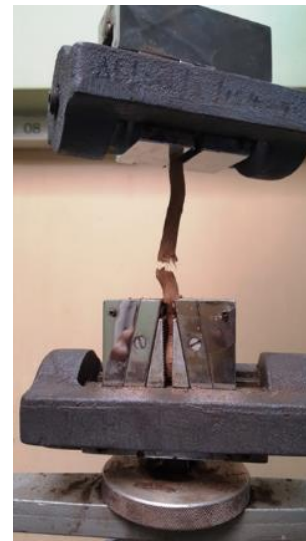
Fig. 3 Root tensile strength testing using Dynamometer
