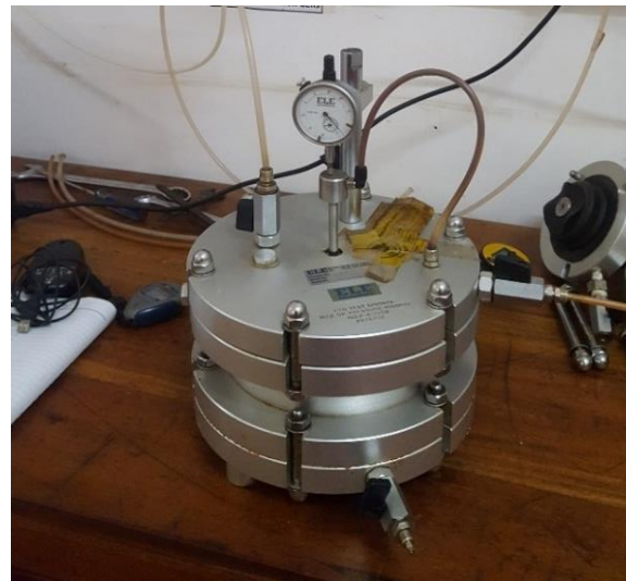
Fig. 6 Rowe cell apparatus used for the study
