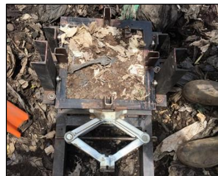
Fig. 4 Specimen prepared for the in-situ testing
