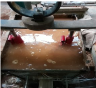
Fig. 4 Saturation of pullout box after the application of back water pressure
