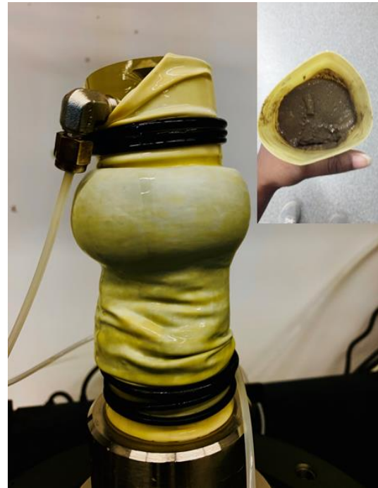
Fig. 7 Fluidized specimen subjected to CSR > CSR_c
