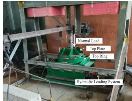
Fig. 2: Large Scale Direct Shear Apparatus.
