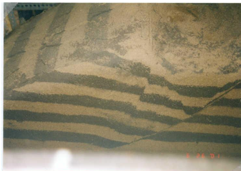
Figure 7 : Failure Surface of the Sand Model without Nails
