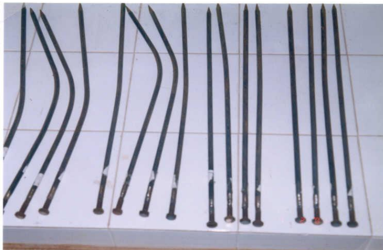
Figure 12 : Bent up Nails Compared with Normal Nails
