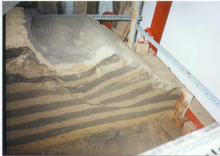
Figure 11 : Failure Surface of the Nailed Sand Model
