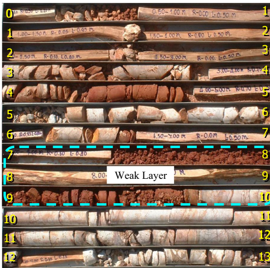
Fig. 15 Core samples showing the weak zone
