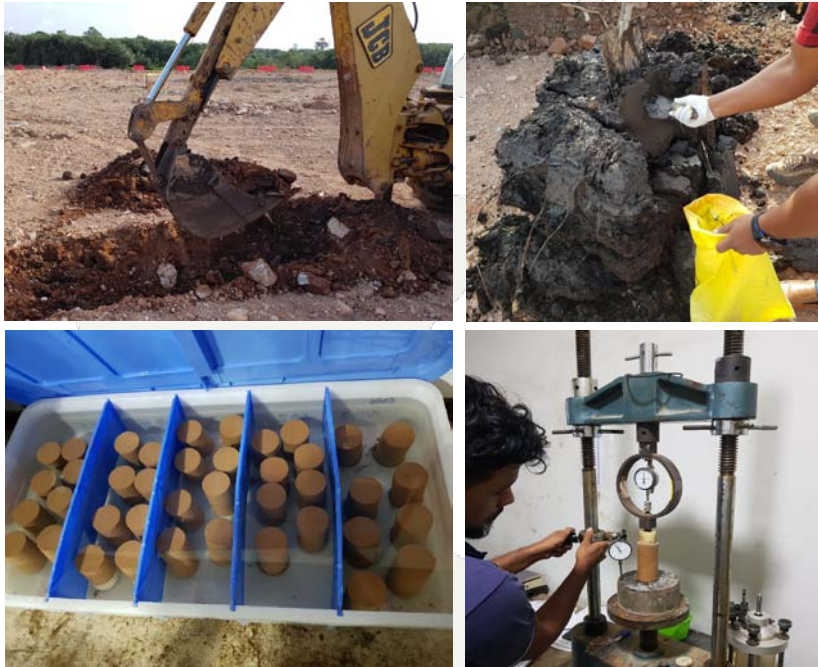
Pre-mixing test for PEAT soil in Sri lanka
