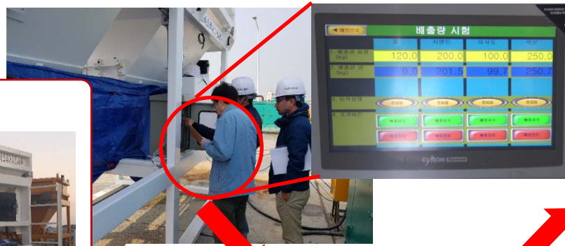
1. Set targeted weight (Ex: Aggregate 250kg)
