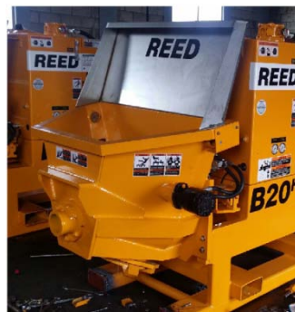
Injection pump (Material delivery)
