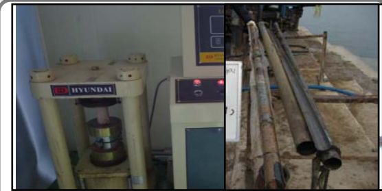
Uniaxial compression test of core
