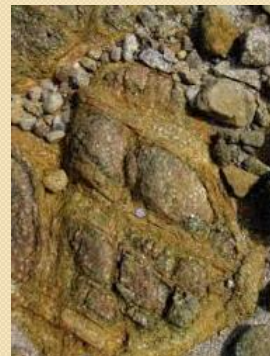
Typical weathering profiles of the bedrock
