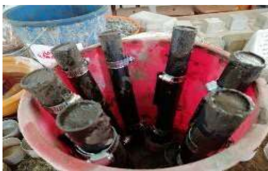
Figure 2 Casted soil-cement columns
