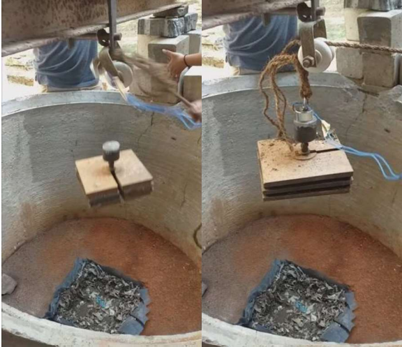
Fig. 3 Free falling of the weight and lifting up by rope
