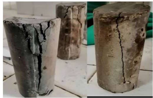
Figure 10 (a) Crack pattern of small cylinders
