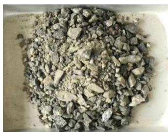
Fig. 1. Crushed stone mix
