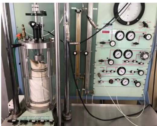
Fig. 4 Triaxial testing of remolded samples
