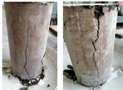
Figure 10 (c) Crack pattern of large cylinders
