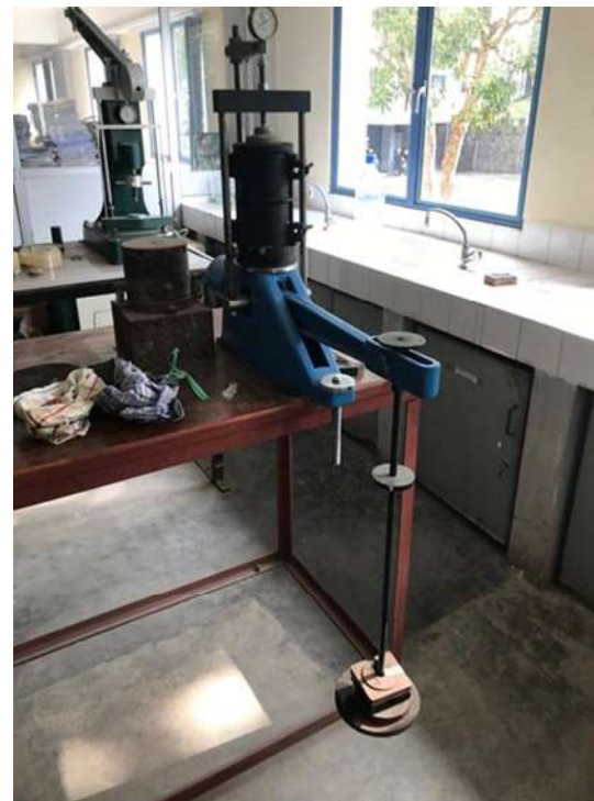
Fig. 3 Modified oedometer apparatus for apply preconsolidation
