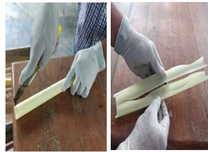
Fig. 1. Splitting of PVC pipes
