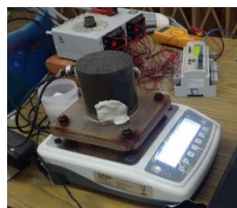
Figure 4: Soil sample connected with tensiometers
