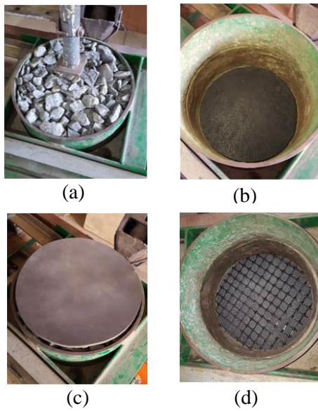
Figure 5 Sample placement; (a) Fresh ballast, (b) UBM at the bottom of the ballast, (c) USP on the top of the ballast and (d) Geogrid on top of UBM
