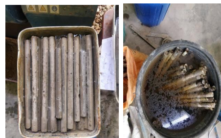
a-Soil cement columns b-Curing process
