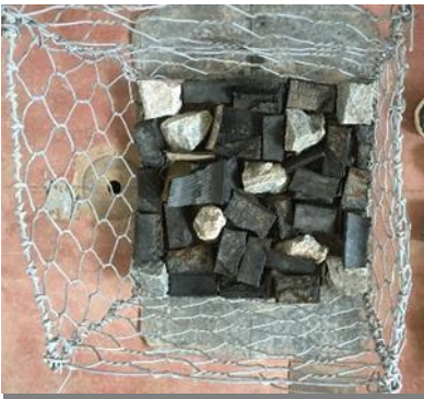
Fig.2 Packing arrangement of shredded tyre and rock for a unit block
