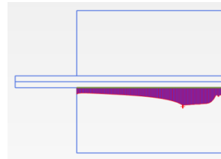
Fig. 9 Variation of shear stress along the nail during pullout
