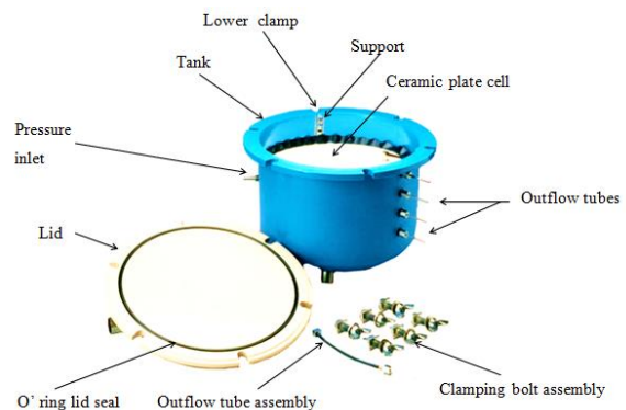
Figure 4: Major components of pressure plate apparatus
