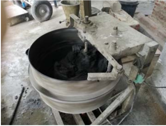
Fig. 1 Mechanical mixing of soil
