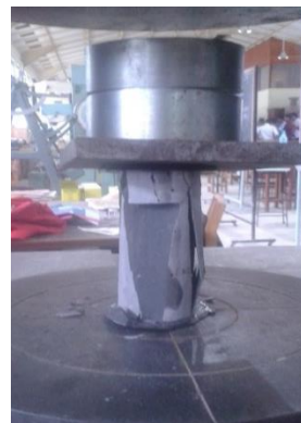
Fig. 1: Sulphur capped sample subjected to Uniaxial Compressive strength test.
