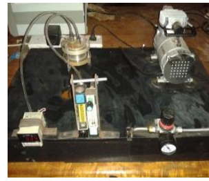
Figure 1- Air permeability Setup
