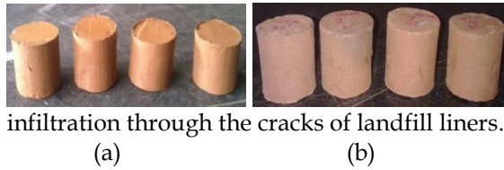
Figure 2: (a) Test specimen after consolidation (b) Test specimen after being oven dried
