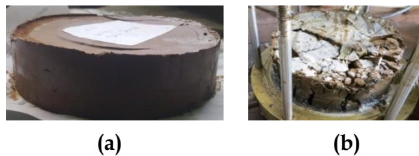
Figure 1: (a) Moragahakanda L1 and (b) water treatment plant sludge consolidated specimens
