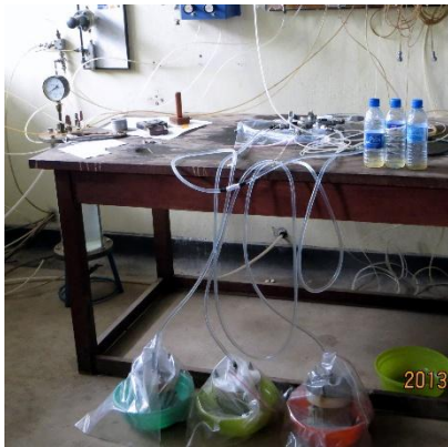
Figure 1: Hydraulic Conductivity Test Arrangement
