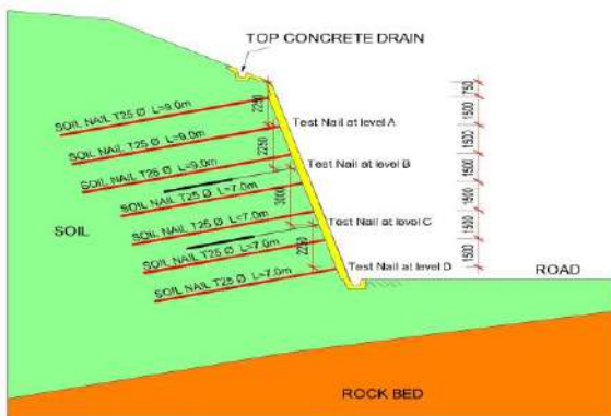
Figure 4: Proposed nailing arrangement
