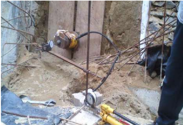
Figure 6: Apparatus used to pull the test nails
